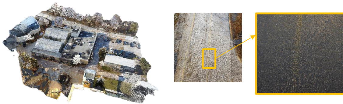
Figure. 9 3D model of UAV and TLS data fusion
