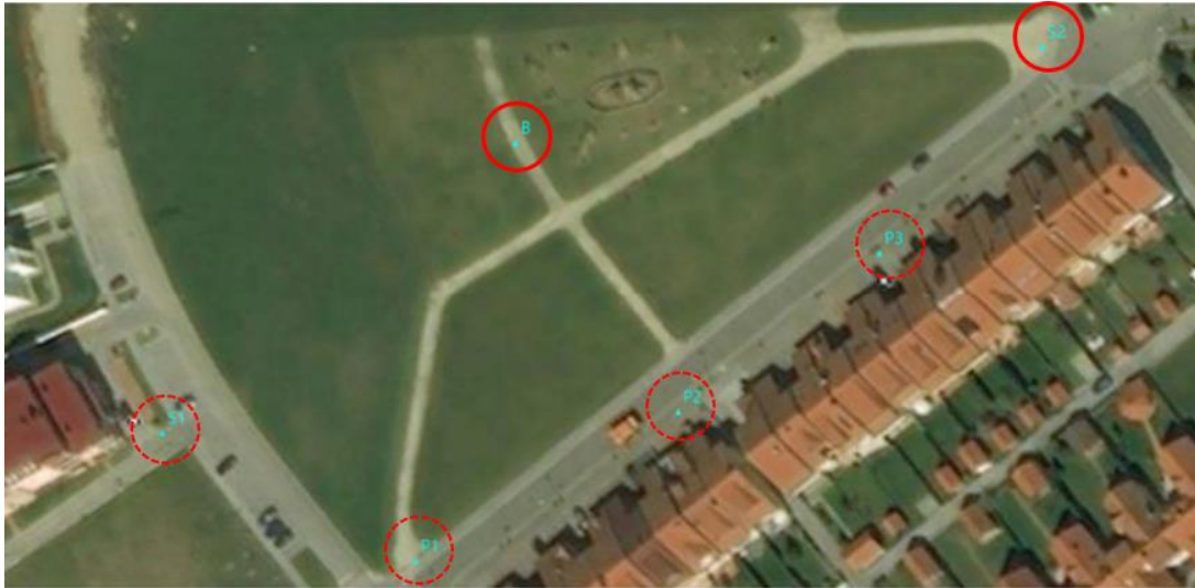
Figure 1. Stations of the geodetic network where the testing took place (with solid circles are marked the station statically occupied with GNSS, with dashed circles those observed with terrestrial methods)
