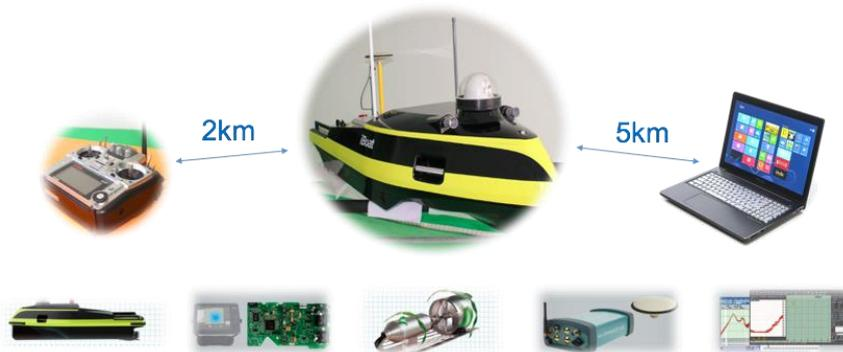
This advanced and autonomous system consists of the vessel body, excellent echo sounding module and positioning module, of course, the data communication system and the controlling system are included.
